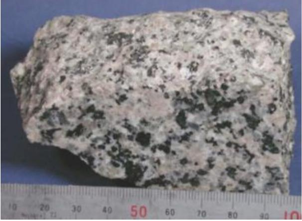
A photograph of a granite rock sample, light-colored with dark mineral inclusions. A ruler is placed below the rock for scale, showing markings from 10 to 100. |
